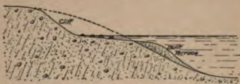
FIG. 257. — Cut and built terrace with boulder pavement shaped by waves on a steep shore formed of loose materials.
